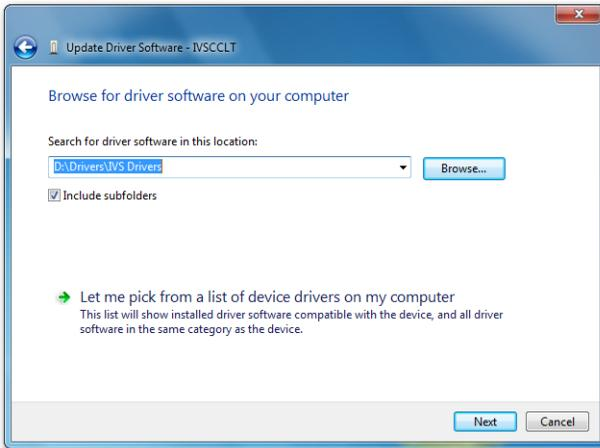
The driver for the Lite Base Station is on the thumb drive that came with the system. Make sure that the thumb drive is connected to one of the computer's USB ports. Next, click on the **Browse...** button to indicate the location where the driver software can be found. They can be found in the IVS Drivers folder, which is in the Drivers folder on the thumb drive.
