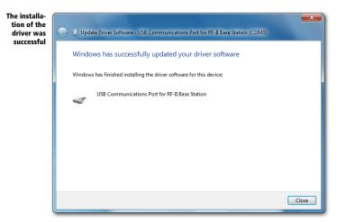
Click on the **Close** button to close the wizard. In the USB Communications Port for RF-II Base Station (COM3) properties window you can see that the device is now working properly.
