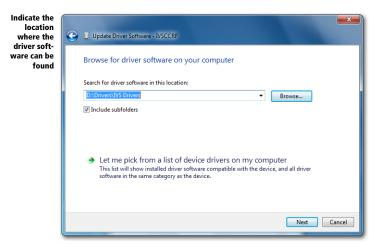
The driver for the RF-II Base Station is on the thumb drive that came with the system. Make sure that the thumb drive is connected to one of the computer's USB ports. Next, click on the **Browse...** button to indicate the location where the driver software can be found. They can be found in the IVS Drivers folder, which is in the Drivers folder on the thumb drive.
